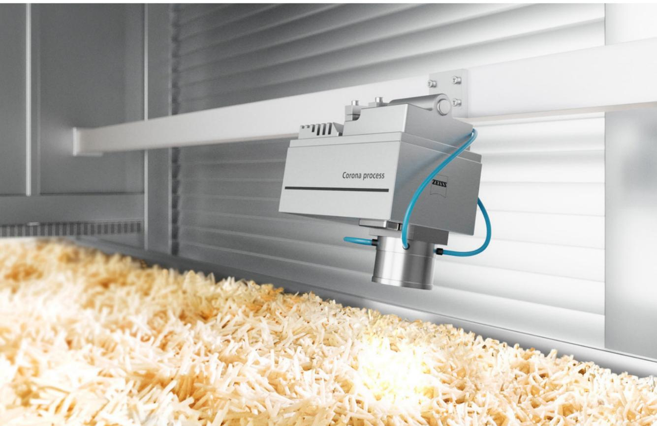
ZEISS Corona<sup>®</sup> process is directly integrated into the production line for in-line measurements. The sensor captures data about constituent elements and the color of potato products on the production line in real time.
