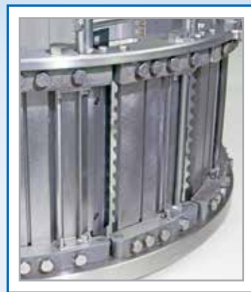
Knife holder, clamp, knife, adjustable gate, and modular block with screws makeup each of the 14 cutting stations
