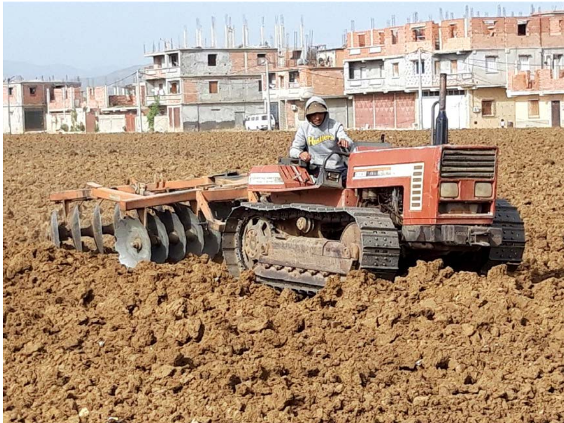
Figure 1. Soil preparation with a disc harrow near Algiers, note the big hard clods.
