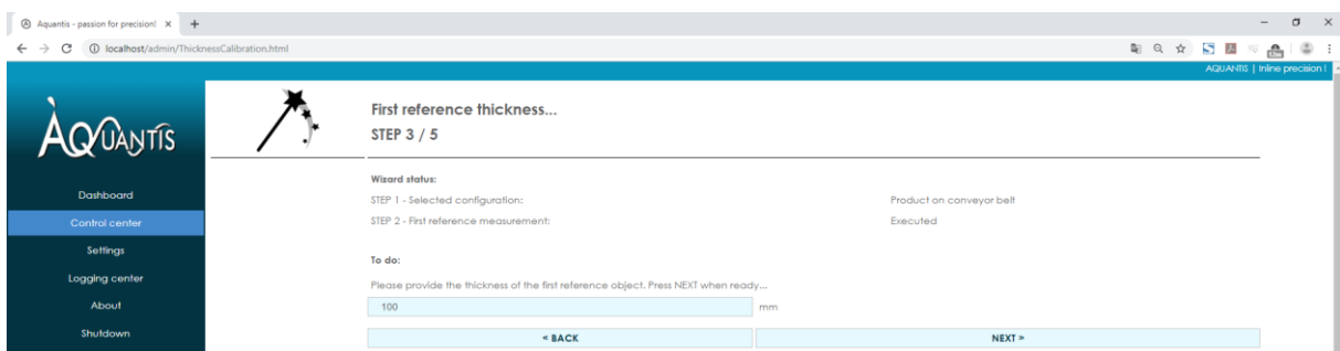
FIGURE 14: THICKNESS SENSOR CALIBRATION WIZARD - THICKNESS INPUT OF REFERENCE 1.
