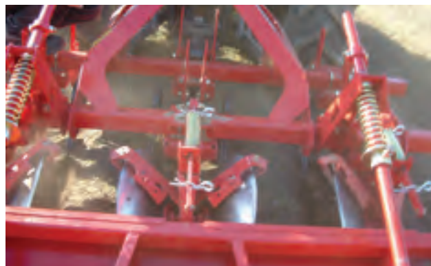
Loosening compaction on the shoulder of the ridge using tines mounted on the front of a rotary hiller also allows greater water infiltration and crop rooting.
