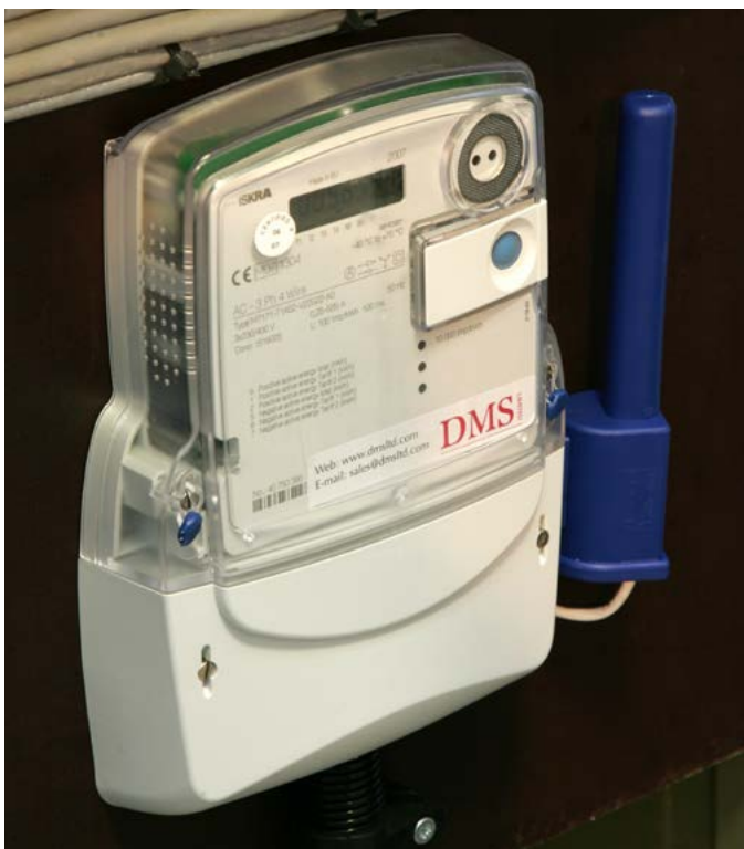
Figure 23. Store-specific smart meter
